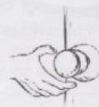
**5. Pulley** – A pulley is a simple machine that uses grooves wheels and a rope to raise, lower or move a load. A wheel with a rope is used to hoist the flag up to the top of a tall flagpole. This simple machine can also be used to help lift heavy objects with less force.
