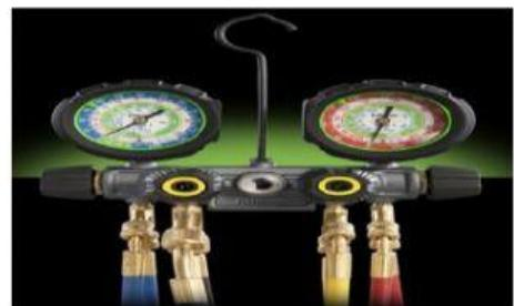
**Connect service hose to the gauge set to the vacuum pump inlet**
