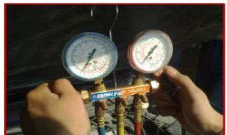
**Connect the manifold gauge hose to low and high side port**
