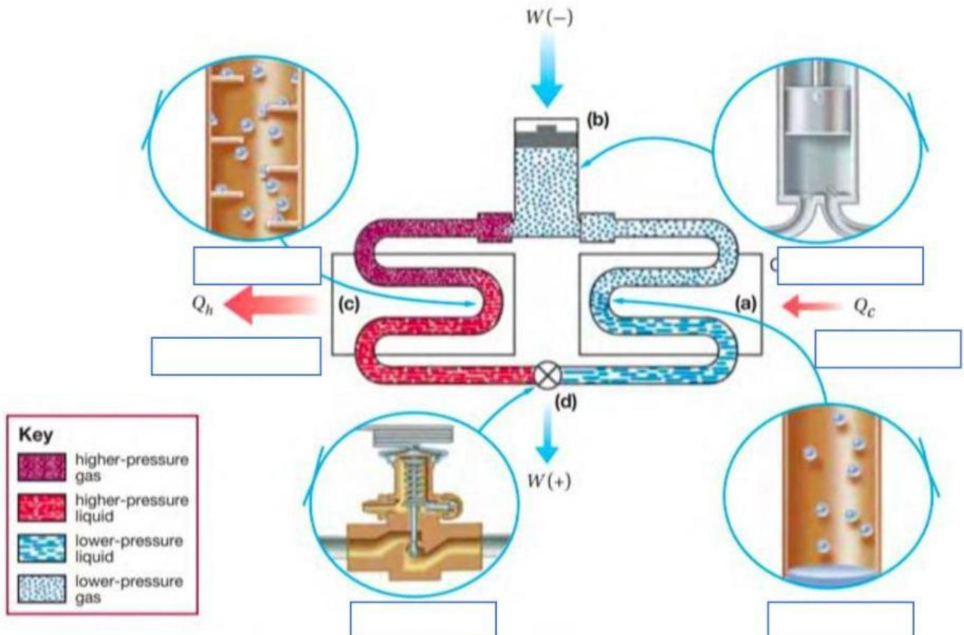
*In each of the four steps of a refrigeration cycle, energy is transferred to or from the refrigerant either by heat or by work.*
