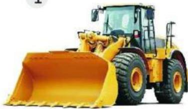
This is used to push large quantities of soil, sand, etc. during construction work.
