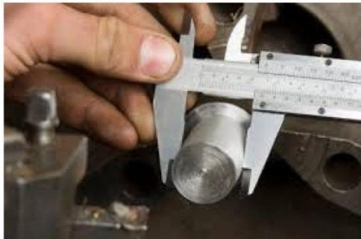
Read the measurement on the main scale.
