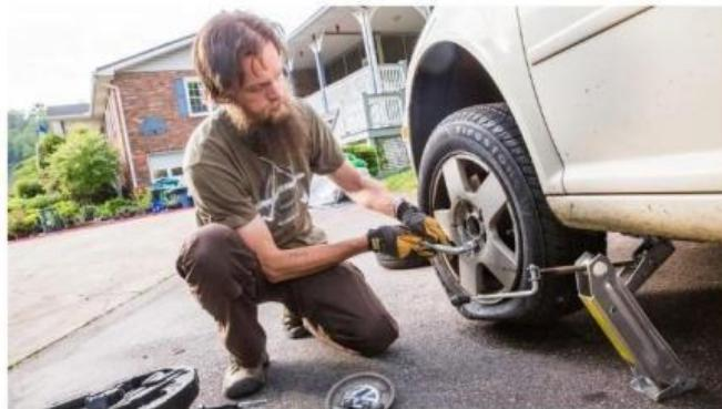
Place the jack under the car and lift the car until the tire is off the ground.
