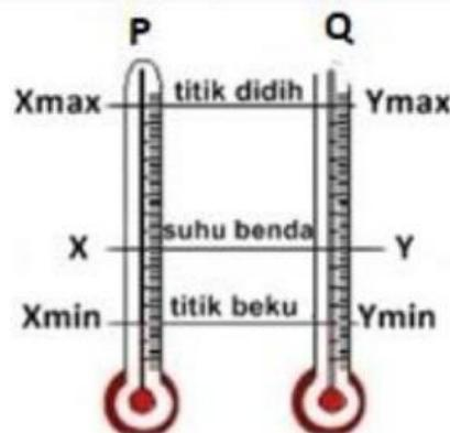
$$\frac{X - X_{\min}}{X_{\max} - X_{\min}} = \frac{Y - Y_{\min}}{Y_{\max} - Y_{\min}}$$
