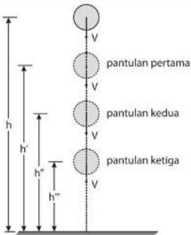
$$e = \sqrt{\frac{h_1}{h_0}} = \sqrt{\frac{h_2}{h_1}} = \sqrt{\frac{h_3}{h_2}}$$
