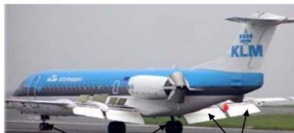
(a) Landing gears and flaps
