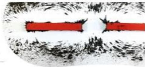
**WE CAN TELL THAT THE MAGNETIC FIELD LINES BETWEEN THE TWO POLES ARE BLENDING AWAY FROM EACH OTHER.**
