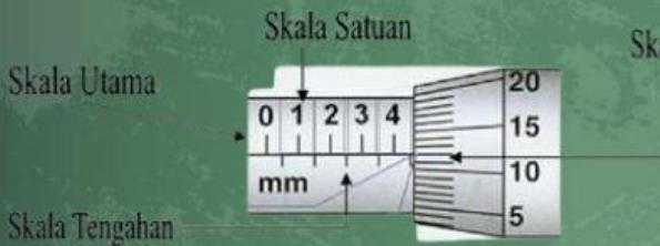
$$\begin{aligned} X &= SU + (SN \times NST) \\ &= 4,5 + (12 \times 0,01 \text{ mm}) \\ &= 4,62 \text{ mm} \end{aligned}$$
