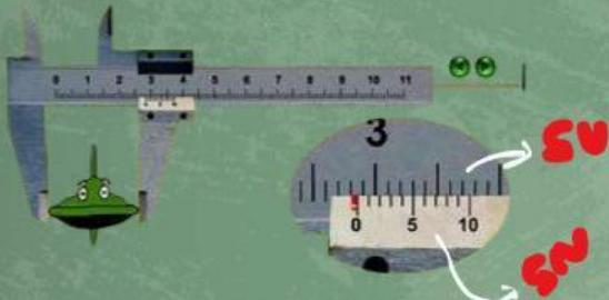
$$\begin{aligned} X &= SU + (SN \times NST) \\ &= 2,8 + (5 \times 0,01 \text{ cm}) \\ &= 2,85 \text{ cm} \end{aligned}$$
