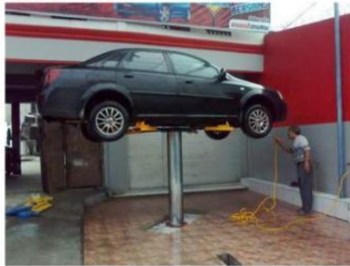
Picture 1. Hydraulic car wash equipment (Source : Tokopedia.com )
