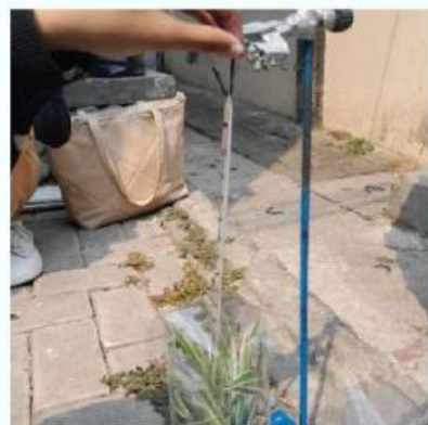
Picture 5. Install the thermometer on the stand and insert the bottom into the container through the square mica hole that has been previously punched
