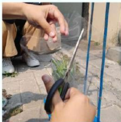
Picture 3. Divide one of the mica into 2 parts with scissors into a square shape and then make a hole
