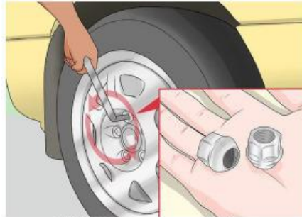
STEP 2: Remove the lug nuts.
