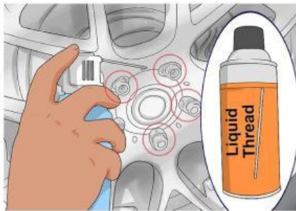
STEP 3: Apply liquid thread to loosen it if need be
