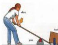
It is made up a long bar that moves up and down over a point known as a pivot.
