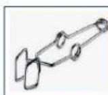
is a clamp used to safely hold a test tube during experiments.
