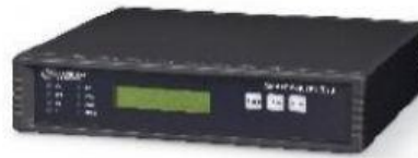
Gambar 1.9 CSU/DSU ( Channel Service Unit/Data Service Unit )
