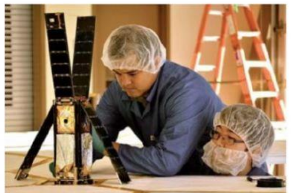
Figure 2. Two engineers work on a cube-satellite that will be launched into space to test the deployment mechanism for a solar sail—the silver folded sheet
