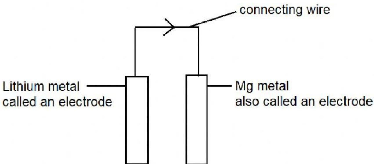
Since Li wants to give off electrons (oxidise) and Mg wants to gain electrons (reduce) It creates a flow of electrons – and thus electricity.
