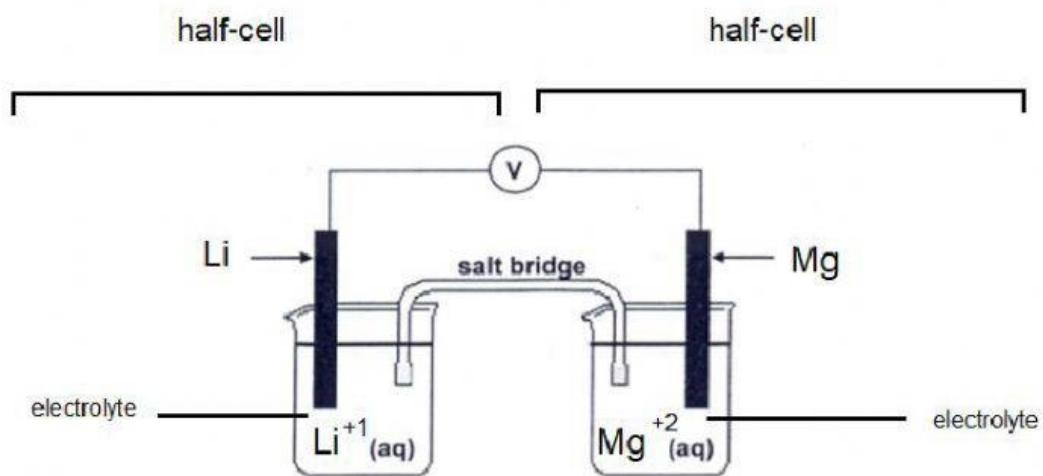
The whole setup is known as a galvanic cell (the basic setup of a battery)
