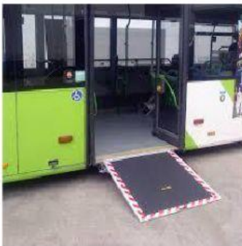
BUS WHEELCHAIR RAMP
