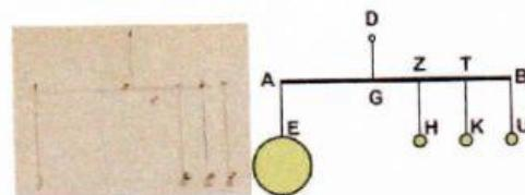
Jika jarak  $AG = 40 \text{ cm}$ ,  $GZ = 20 \text{ cm}$ ,  $ZT = 20 \text{ cm}$ ,  $TB = 20 \text{ cm}$ , dan massa  $M_E = 10 \text{ kg}$ ,  $M_H = 2 \text{ kg}$ ,  $M_U = 2 \text{ kg}$ ,  $g = 10 \text{ m/cm}^2$ , maka massa  $M_K$ , agar sistem setimbang di titik  $G$  adalah...
