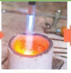
▲ 2. MELTING The heat is carefully controlled to make the ore melt but not turn to vapour.
