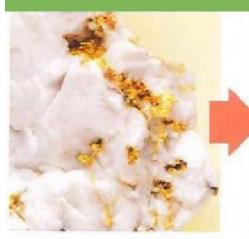
▲ 1. ORE Sometimes small pieces of metal can be seen in the ore, such as these flecks of gold.
