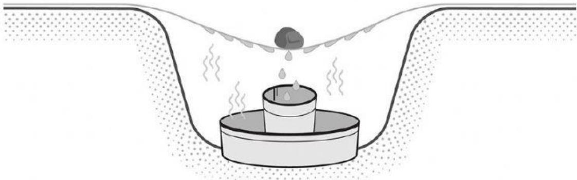
The hole is then covered with a plastic sheet, as this kind of material will trap rising water as it evaporates.
