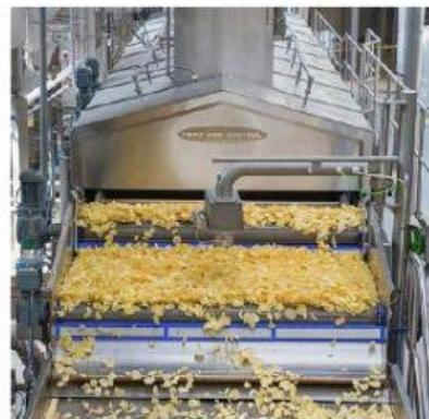
\_\_\_\_\_ may be mixed with the salt or dusted or sprayed onto the crisps in rotating drums. Finally, the crisps are cooled and packed.
