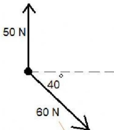
Break any forces at an angle into components first
