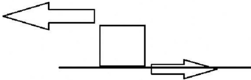
The **frictional force cannot exceed the applied force** on the object.
