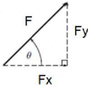
If we are given the force  $F$ , then we can calculate the horizontal and vertical component of that force using Trig.
