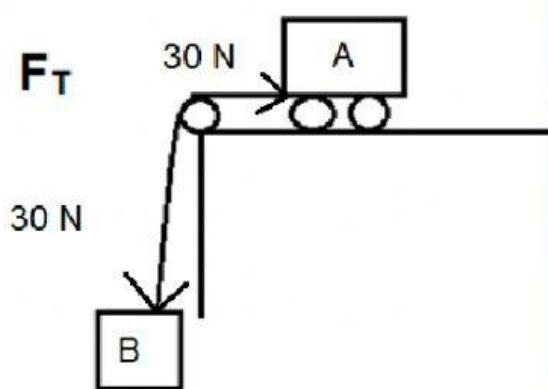
The tension pulling in both directions will be the same within the same rope. For example if the tension in this string is 30N then the tension force trying to pull box A down is 30 N and the tension trying to keep box B from dropping to the floor is also 30N
