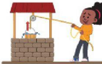
Pulley - Water Well
