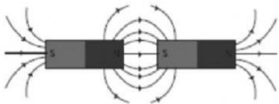
These two bar magnets are \_\_\_\_\_ each other. The magnetic field lines go from the \_\_\_\_\_ pole of the first magnet to the \_\_\_\_\_ pole of the other.
