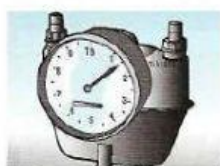
gas flow meter
