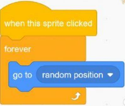
A Scratch script consisting of a yellow "when this sprite clicked" hat, an orange "forever" control loop, and a blue "go to random position" movement block.                                             |                |
