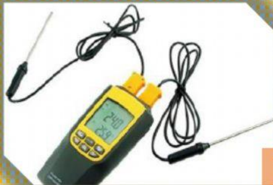
Gambar 6 Termometer termokopel Sumber: www.digital-meter-indonesia.com
