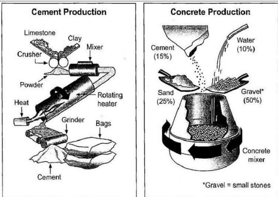
The diagram above shows the stages and the equipment used in the cement making process and how cement is used to produce concrete. Write a description of the process. Use at least 150 words.
