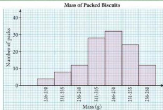
A quality control supervisor wants to determine whether the batch of biscuits produced by the packaging department follows the specifications of the standard mass. The histogram shows the mass of packed biscuits in a few sample tests.
