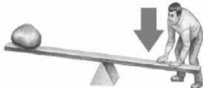
With the fulcrum far away from an object, the object is harder to lift, but it can be lifted higher.
