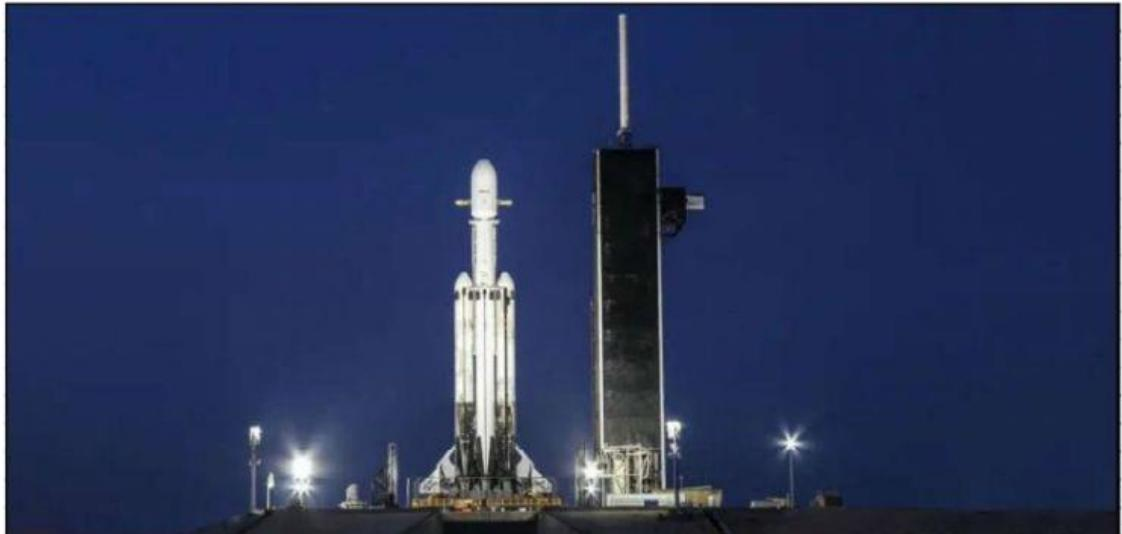
Falcon Heavy is the world's most powerful rocket. It was first launched into space on February 6, 2018 and has been launched two more times since then. Falcon Heavy is a rocket that stands 70 m tall and weighs 1,420,788 kg. Regarding its structure, the first stage has three parts, or cores, each with nine identical rocket engines, making 27 engines in all. Each core is a Falcon 9, an earlier SpaceX rocket. The
