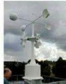
Anemometer (Wind speed)
