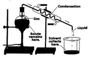
When a solution is distilled, both the solvent and the solute can be recovered. The solution to be separated is heated. The solvent evaporates and forms a gas. The gas moves through a tube called a condenser. The condenser cools the gas back to a liquid. The liquid drips into a container. The solute remains in the original container. Both the solute and the solvent are recovered.
