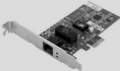
Each computer contains a NIC. Today this card comes with an inbuilt component of the computer motherboard. It is a must to have a NIC to connect to the internet. The main purpose of NIC is to format the data, send the data, and receive the data at the receiving node.
