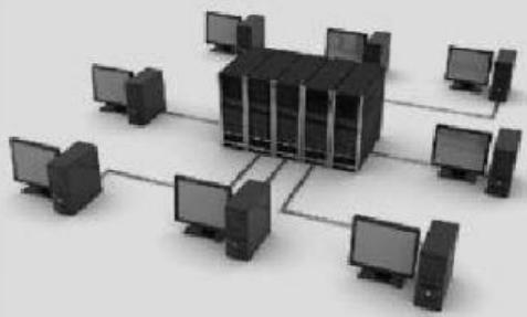
The computers are the clients of the network. It can receive and send data to another computer. The above diagram shows several client computers connected to servers.
