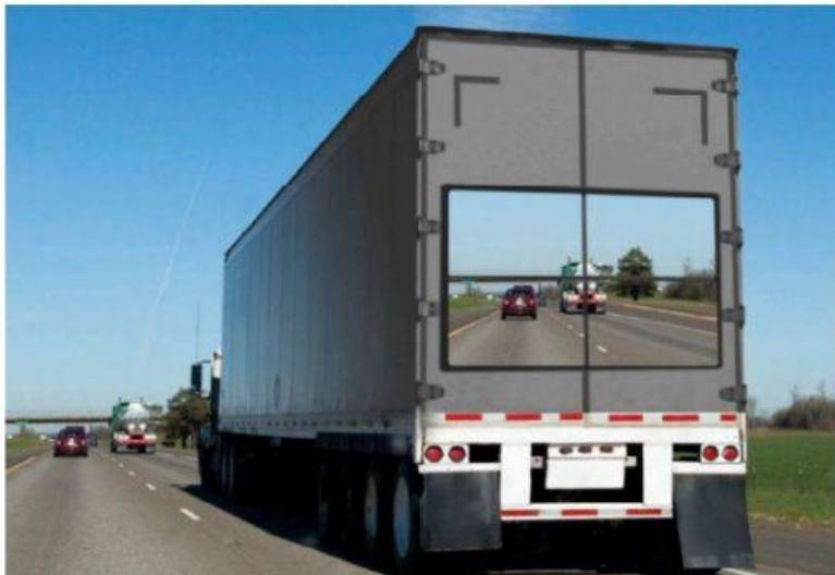
Drivers often find it difficult to get past a large truck safely because the truck blocks the view of the road ahead. One possible solution is to put a camera on the truck's hood that sends images to a screen on the truck's back. Drivers behind the truck can then see what's ahead of it and decide when it is safe to try to pass.
