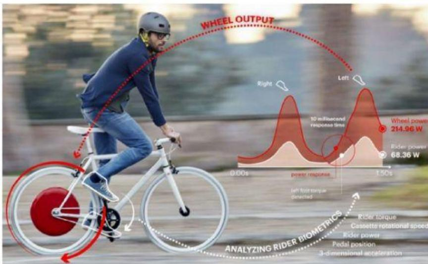
The Copenhagen Wheel is designed to make it easier to pedal a bike by increasing the power supplied to the wheels. The red wheel hub contains an electric motor and battery that help amplify a rider's
