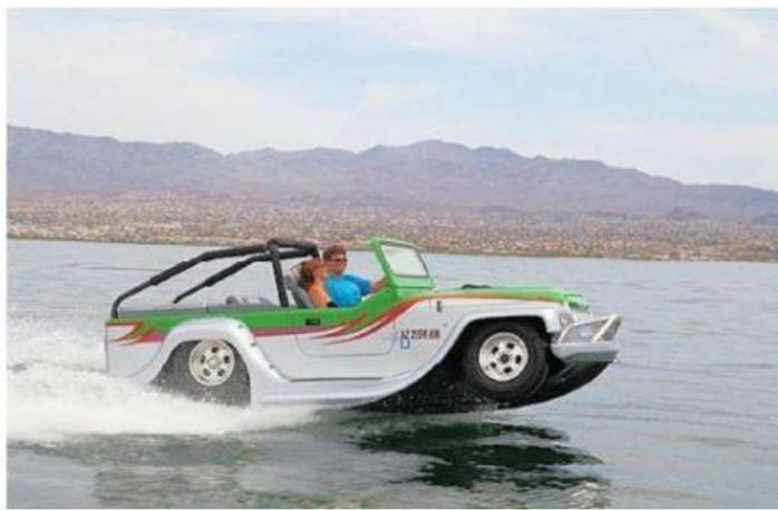
Deep water defeats most cars, but the WaterCar Panther keeps going. The Panther is an amphibious car, equally happy on land or in water. In water, the driver pulls a lever to activate a waterjet at the back of the car and pushes a button to raise the wheels. The waterjet propels the car. The Panther is fast enough to pull water skiers.
