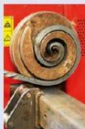
Metal changes shape when a  is exerted. The deformation is  as the metal bar does not return to its  shape.
