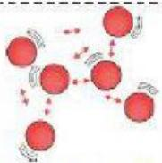
The vibrations pass from particle to particle.
