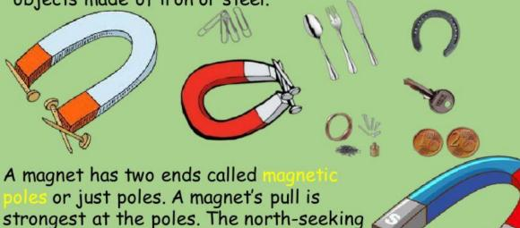
At times magnets pull toward each other, but at other times they push away from each other. This is a magnetic force caused by magnetic fields. A magnetic field is the space all around a magnet where the force of the magnet can act.
