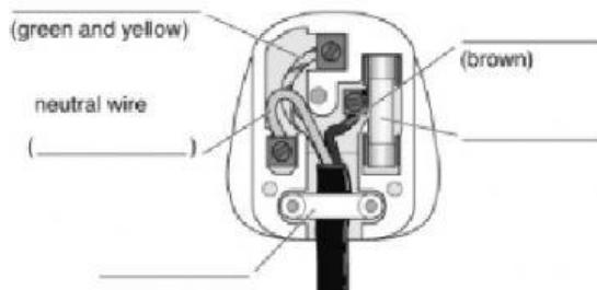
A hairdryer is connected to the mains supply using a plug. When the hairdryer is working correctly the current is 4 A. What will happen if something goes wrong and the current is 6 A?
