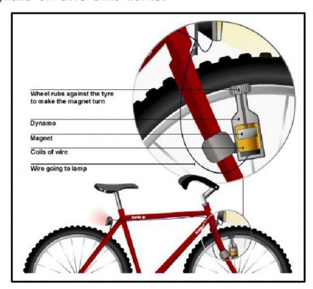
an electric current is produced. the bicycle wheel turns the dynamo wheel. the current travels along the wire and the light switches on.
