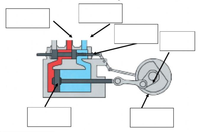
The Flywheel: This is turned by connecting rods through the movement of the piston.
