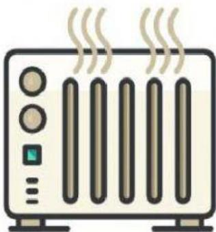
A radiator puts warm air out at the top and draws in cooler air at the bottom
