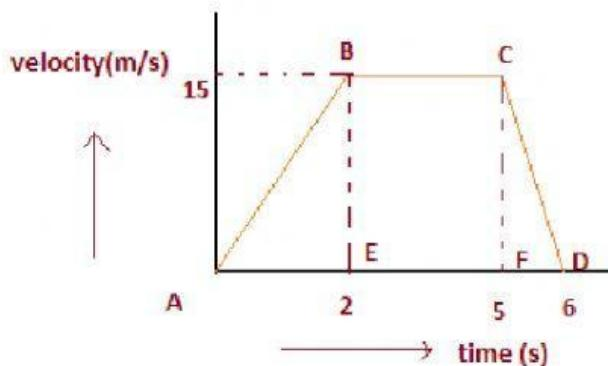
What is the distance travelled by the SUV in first 2 seconds?
