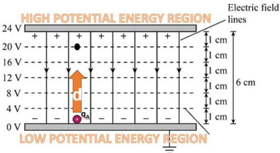
The picture above shows a positive test charge,  $q_A$  positioned at a certain location in the electric field between the two plates. Its movement to the black point is represented by the displacement ( $d$ ).
