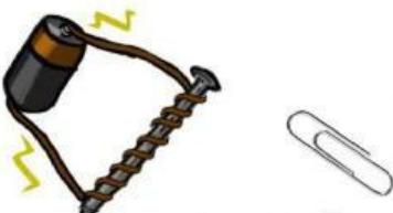
A student moves a paperclip closer to an electromagnet and observes it being pulled more strongly.
