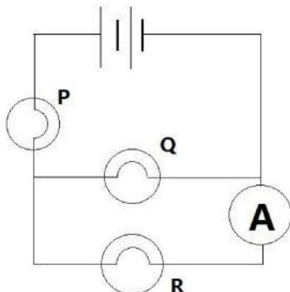
21. Figure above shows a circuit that a student set up, using identical bulbs, P, Q and R. After some time, bulb Q fuses. Which of the following will happen?
