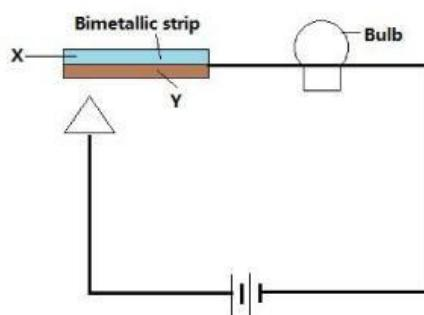
15. Figure shows a model of an automatic fire alarm. Which of the following is true of the automatic fire alarm?
